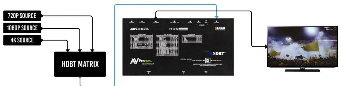
THE AC-EX70-SC2-R CAN GIVE THE SINK ANY RESOLUTION FROM 480P TO 4K 60 NO MATTER WHAT THE SOURCE IS OUTPUTTING
