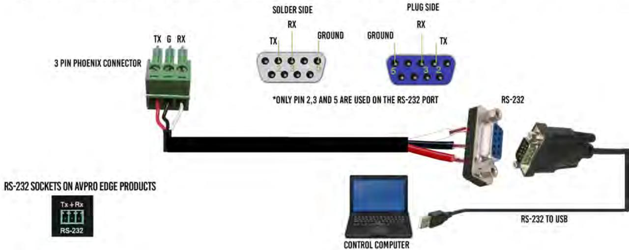
You can send serial commands in the 3-Pin port or the Micro USB port
