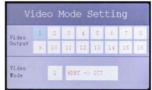
**\*\*NOTE: ONLY THE ODD NUMBERED HDBaseT PORTS CAN BE DOWNSCALED\*\***
