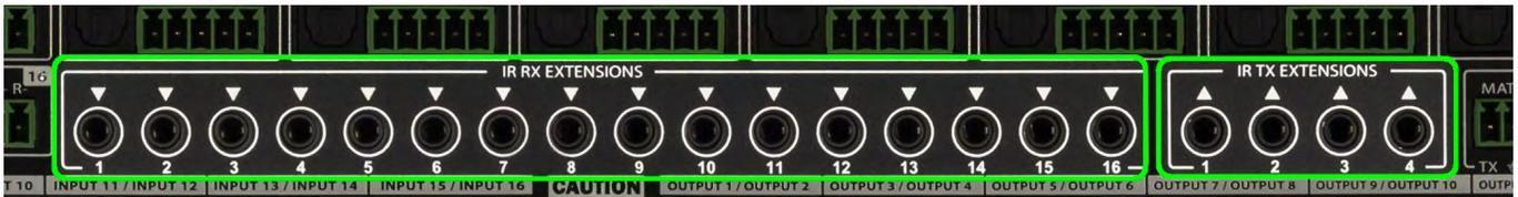
The "IR RX EXTENTION" and "IR TX EXTENTION" ports on the back of the Matrix are designed to be directly connected to a control system. They are not designed to be used with IR Emitters/Receivers.
