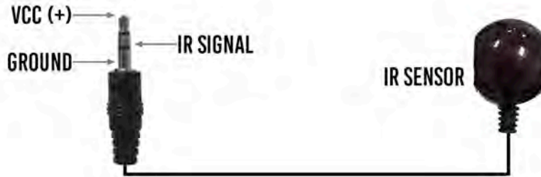
IR IN w/ Receiver Eye ("IR-EYE" MODE)
