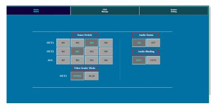
SENSE SWITCH: USE THIS AREA TO ROUTE INPUTS TO OUTPUTS
