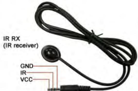
Figure 4 ~ IR Extension Cable
