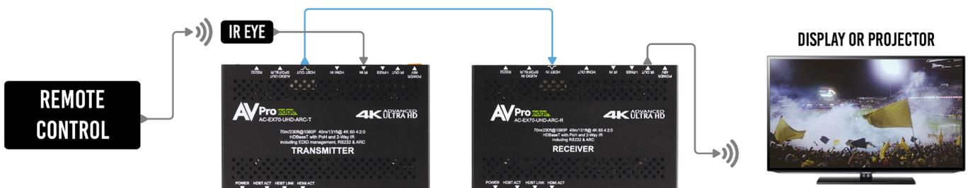
In the example below a control system is plugged into the "IPASS" port of the HDBaseT Transmitter with a 3.5mm mono cable, and a IR Emitter is plugged into the "IR OUT" port of the HDBaseT Receiver. This allows you to send an IR signal from a control system down the category cable to the sync (RX) and control the display.
