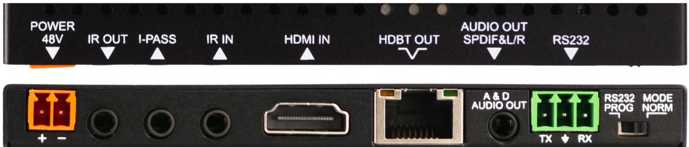
**POWER 48V** - 2 Pin terminal connector. You can power at either the Transmitter or the Receiver. Power will be provided automatically over the Category cable to the other HDBaseT unit.
