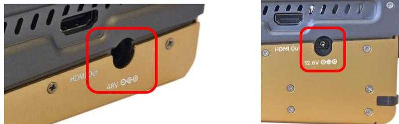
Figure 14: MS103TDs and MS104B Input Powering Sockets
