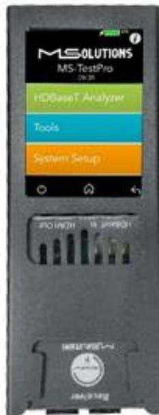
**Figure 1: The MU-M4SOL HDBaseT Test Device**
