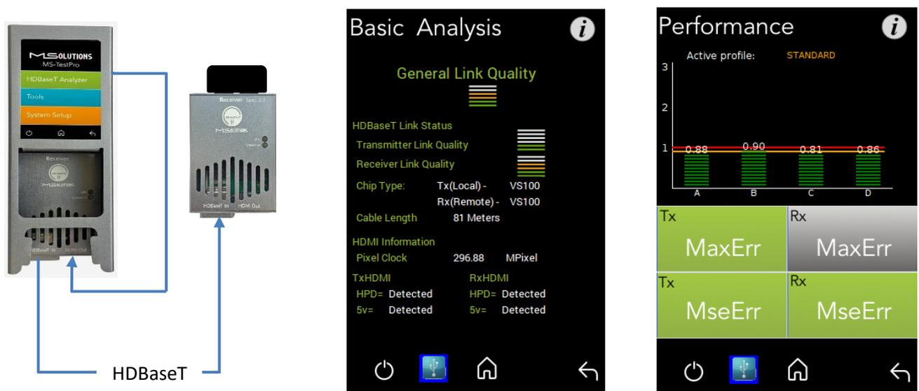
Figure 143: Cable Test Setup
