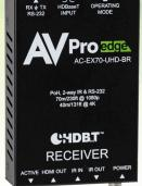
This basic HDBaseT wall plate transmitter/receiver kit is a cost effective HDMI extension product from AVPro Edge's ConferX line-up. This extender kit is able to send a 4k signal 40 Meters and a 1080p signal 70 meters using CAT6a with HDBaseT technology.
