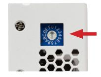
USE A FLATHEAD SCREWDRIVER TO TOGGLE BETWEEN DIFFERENT PRESET EDIDS BY TWISTING
